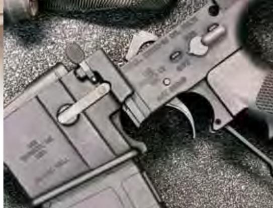
To remove the magazine well you need to unsnap the trigger guard then depress the magazine release and lift the magazine well straight up and off the receiver.
