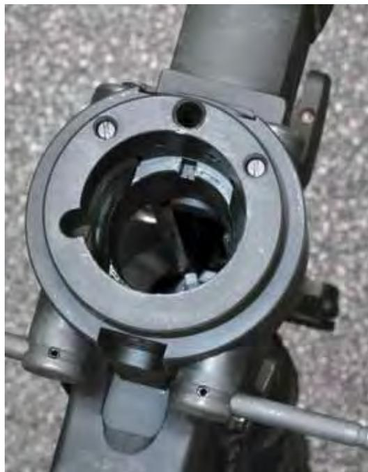
With the handguard removed (four screws) you can see the two locking pieces operated by the two rotating levers. These securely lock the barrel into place.
