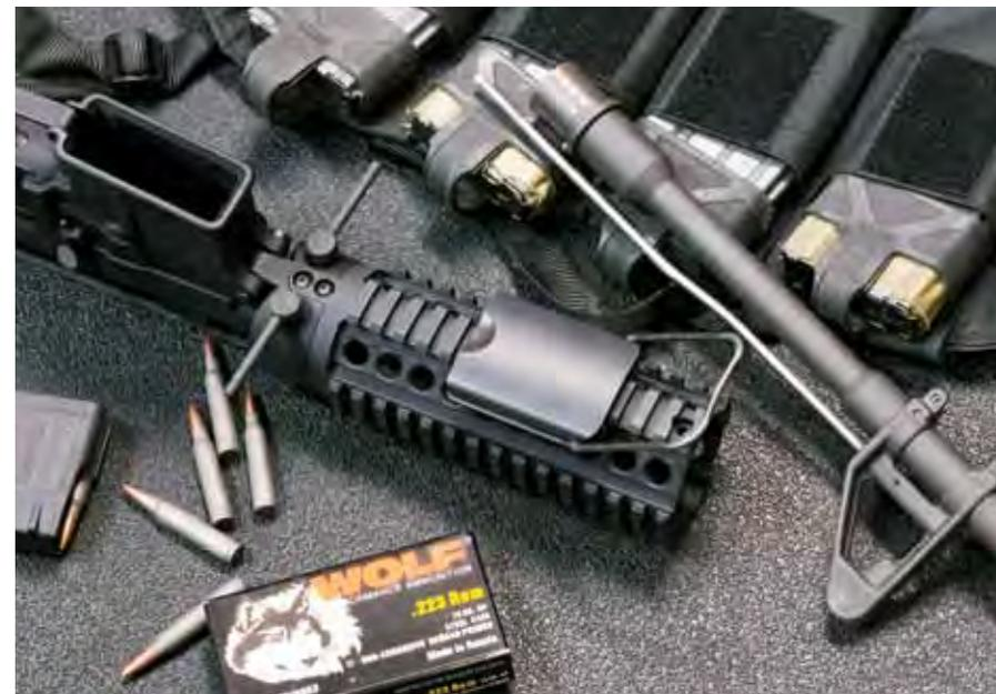
Standard AR-15 barrels can be installed or removed in a matter of seconds with no tools required. MGI's system is not only simple to use but has been in production for years.
