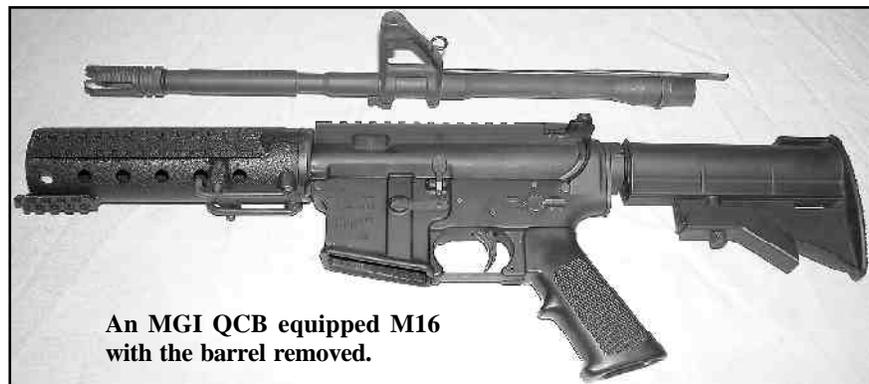
**An MGI QCB equipped M16 with the barrel removed.**
