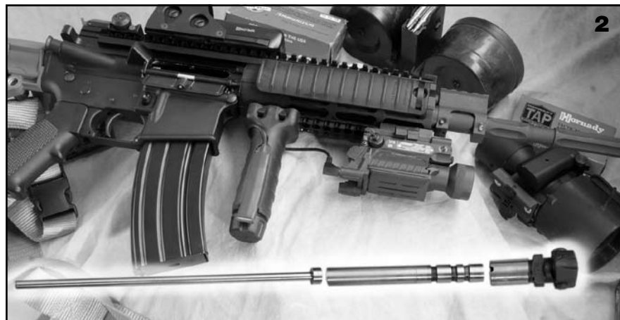
The POF Gas Trap Carbine replaces the direct impingement gas AR gas system with a piston and operating rod, enhancing reliability and operability.
